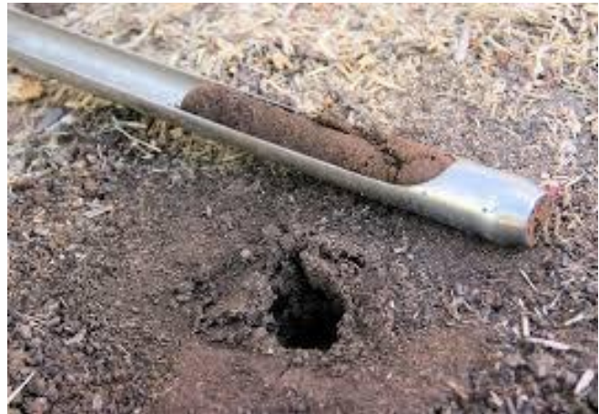
Figure 1. Examples of a soil probe and how it looks after pulling a core.
